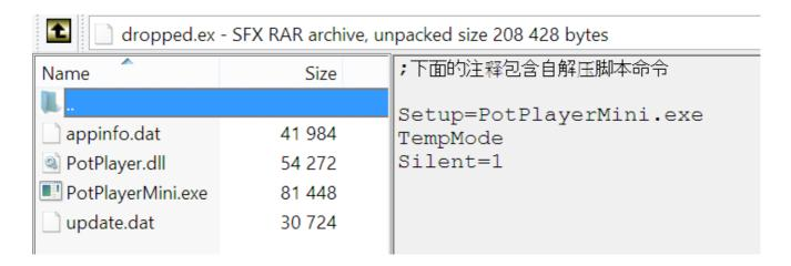
The dropper installs four files in the system. The "Appinfo.dat" file launches "PotPlayerMini.exe", monitors the memory periodically with the GlobalMemoryStatus API function and writes the results to "C:\windows\memstatus.txt"
