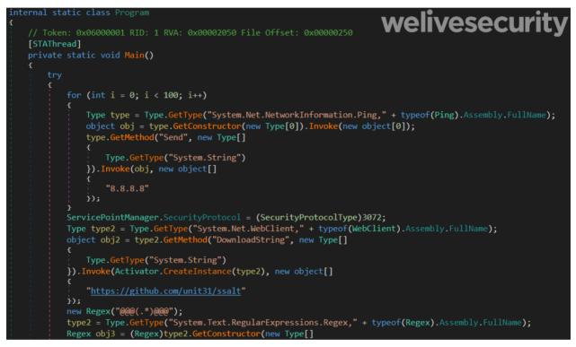
Figure 7. .NET module responsible for downloading and executing a payload stored on github.com
