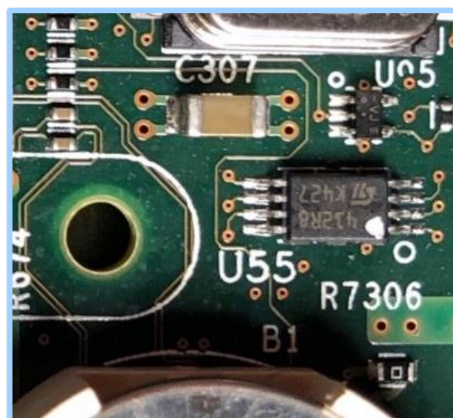
Figure 9. U55, a I 2 C EEPROM, ST p/n M24512 marked 412R8 as found in the Counterfeit A unit.
