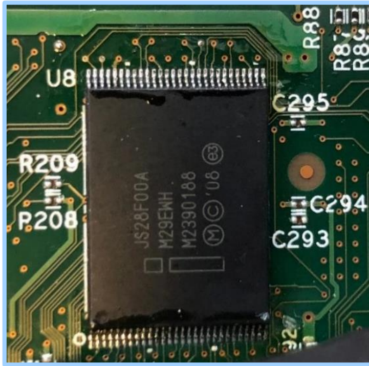
Figure 7. U8, an 1Gbit NOR Flash. PCB rework evidence on the Counterfeit A unit: soldering flux residue on and around the Flash IC is present.
