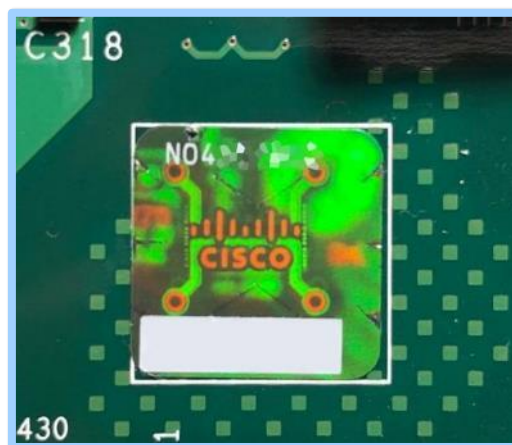
Figure 3. Legitimate holographic sticker which was absent on both counterfeit units.
