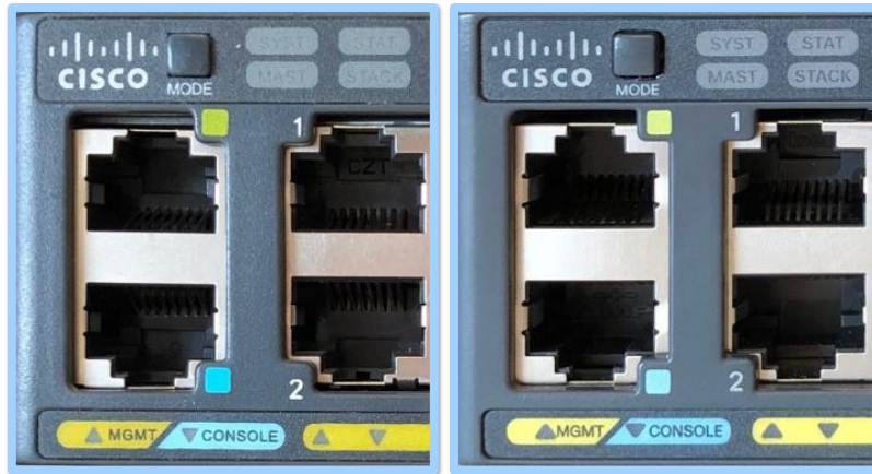
Figure 2. The mode button’s shape is slightly different. The square next to the management port is greenish on the counterfeit switch. On the genuine device, it is bright yellow.
