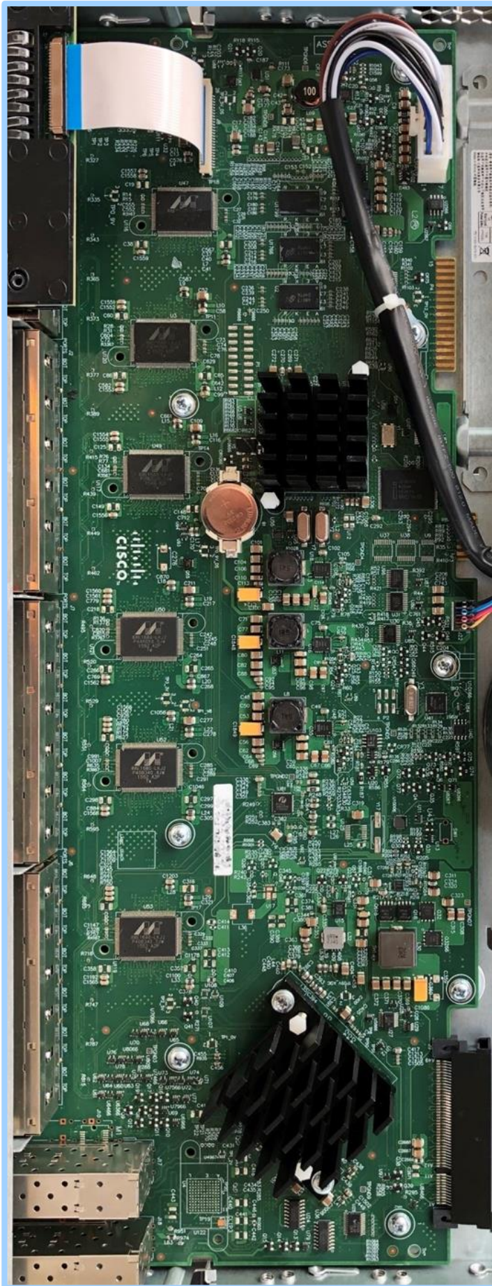
Figure 6. Counterfeit B, internal view.
