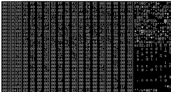
Figure 8. The decrypted format.cfg shellcode; strings with file names and rundll32 command are visible
