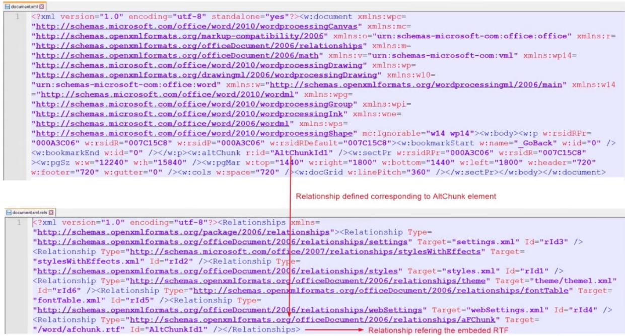
Figure 2: AltChunk element and its corresponding relationship
