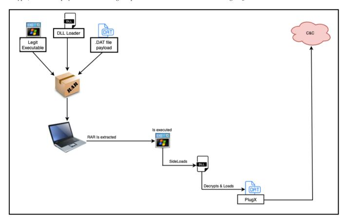
Figure 5 - PlugX side-loading execution chain
