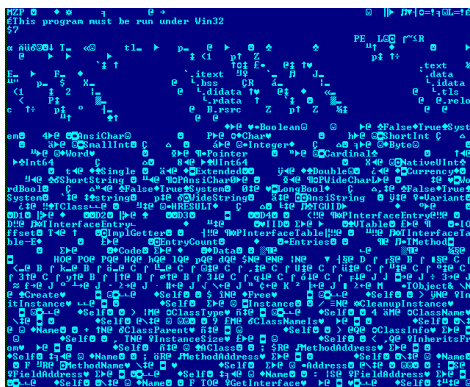
Figure 12. A simple XOR decryption revealed a hidden PE file
