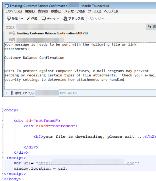
Figure 3. Sample spam email sent on June 13 (top), and screenshot of code showing how the HTML file downloading a malicious document (bottom)
