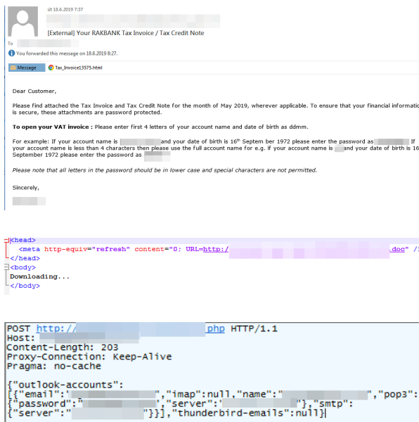
Figure 5. A sample spam email from the campaign observed on June 18 (top); snippet of code showing the malware-embedded .doc file that will be downloaded (center); and snapshot of email credentials being stolen (bottom)
