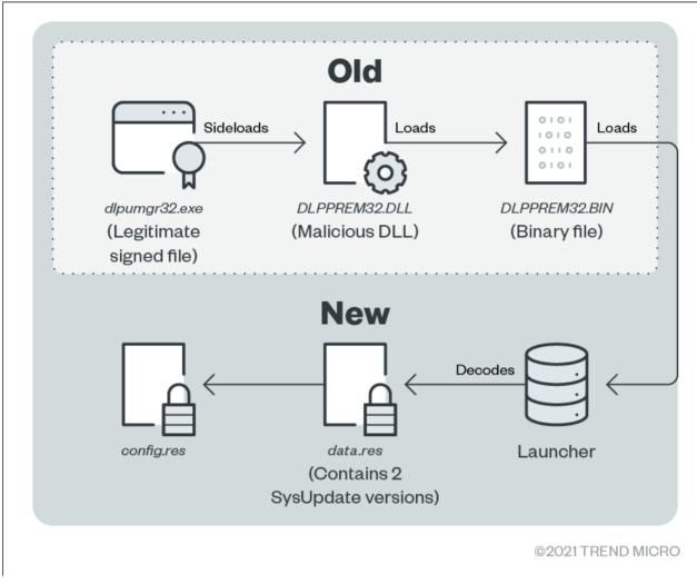
Figure 1. The old and new SysUpdate infection chains
