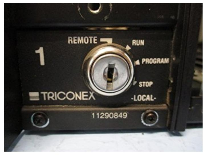
Figure 3: Triconex Key Switch ( source)
