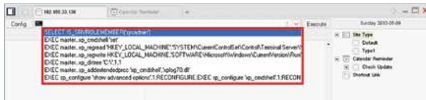
Figure 12: China Chopper's database management feature lets users interact with a database and even provides helpful prepopulated commands
