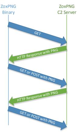
Figure 1: Communication Pattern between ZoxPNG and its C2 Server
