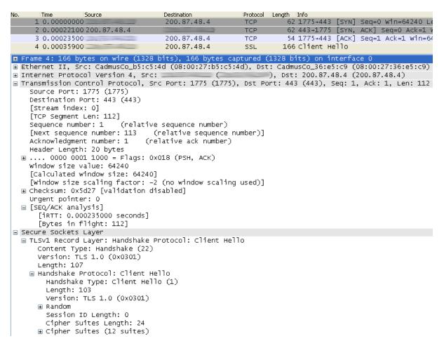
Delving into the disassembly behind the malware we can see that this SSL handshake is clearly faked and generated using hardcoded values within the malware.
