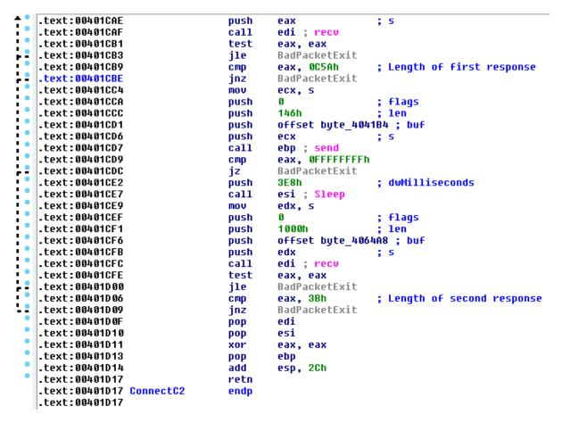
The encoded MAC address is also sent to the command and control server. It is likely that the attacker's use this value to identify unique victims. Once the connection has been established command and control can take place.
