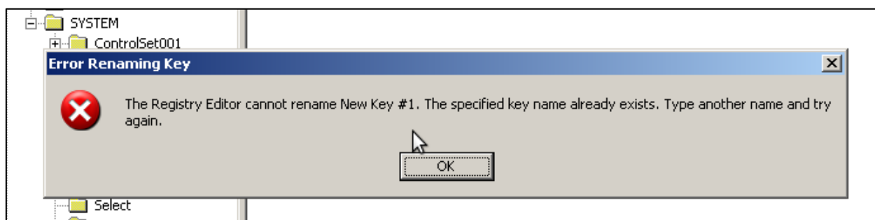
Rootkit detection method - registry key renaming fails if the key already exists.
