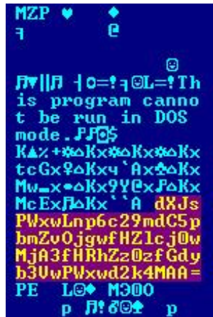
Encrypted settings in the header of malicious executable
