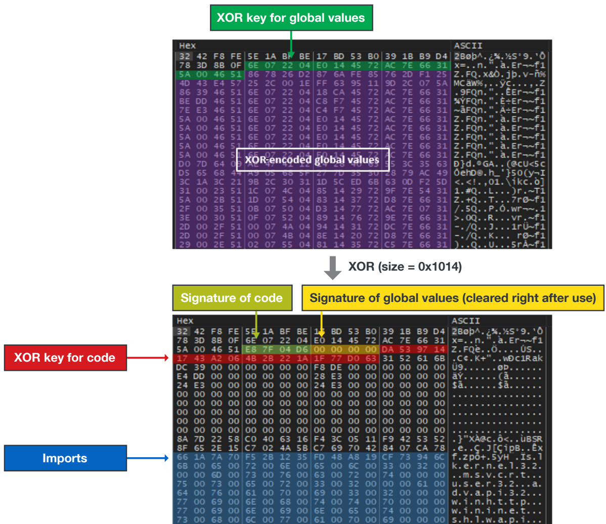
Figure 41. ScrambleCross using a 16-byte XOR to decode its functions and global values
