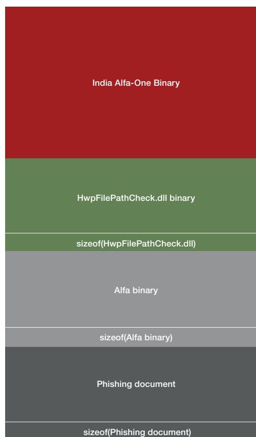
Figure 2-1: Payload File Stacking within IndiaAlfa-One Samples
