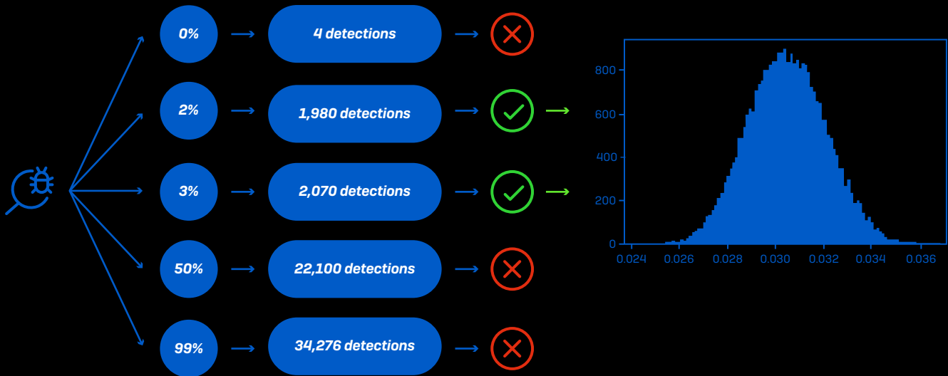
Fig. 28. Propose a malware rate, sample, see if the simulation matches observed reality, tally the rates that do, and repeat. Source: SophosAI.
