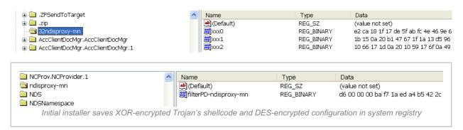
The installer creates the corresponding autostart service and registry keys. The "Altitude" registry value (unique ID for the minifilter driver) is set to 321 000, which means "FSFilter Anti-Virus" in Windows terms:
