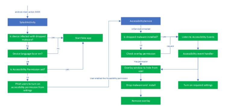
Figure 2: Execution flow of the dropper.
