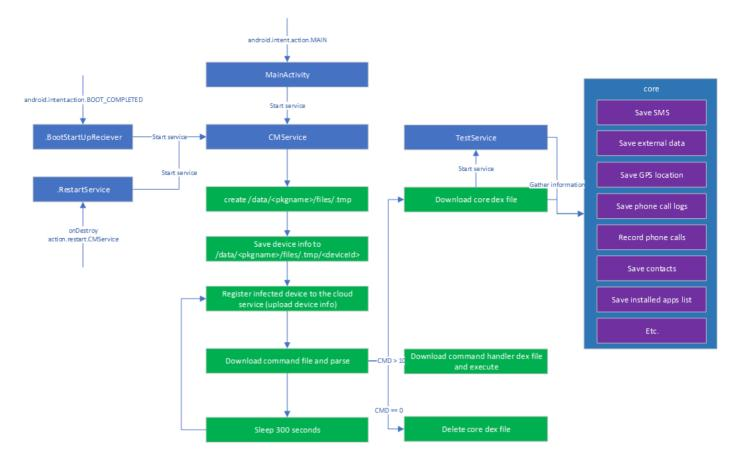
Figure 3: Execution flow of the Trojan.
