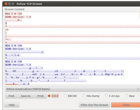
FIGURE 2: Malicious traffic disguised as legitimate Windows Messenger traffic
