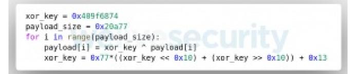
Figure 3. Pseudocode of the payload decryption loop
