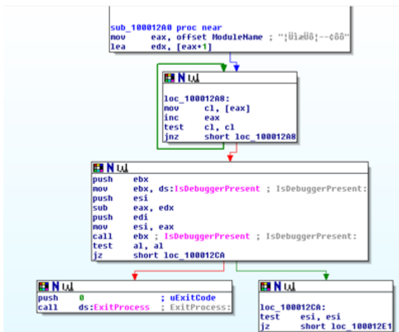
Figure 19. The anti-debugging feature in payload32.dll.
