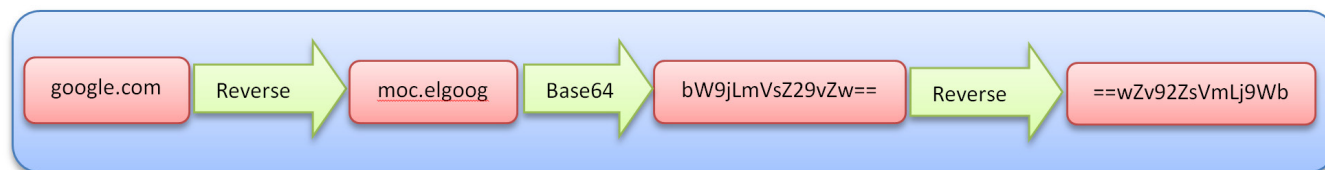
Figure 5 - Communication encoding scheme
