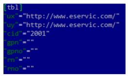
The original module configuration resource is empty - the injector module just patches this resource, replacing the configuration with its own. In the configuration block, "**ux**" and "**uy**" are the C&C servers, "**Cid**" is part of the connection query and seems to be a client ID.
