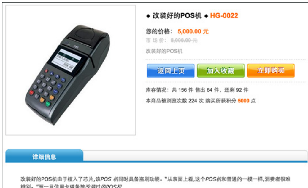
Figure 9: PoS skimmers are sold for RMB 5,000 (~US$788) each on lzise.com; the site is run by a cybercriminal who specializes in selling customized PoS terminals that look no different from those that have not been tampered with, but come with a special chip that allows criminals to authorize otherwise unauthorized purchases
