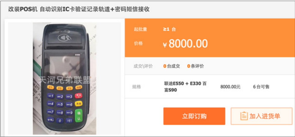
Figure 10: PoS skimmer with an SMS-notification feature sold for RMB 8,000 (~US$1,261) on 1688.com; the device has been modified to allow cybercriminals to instantly receive credit card numbers (including card verification values [CVVs]) via SMS when used
