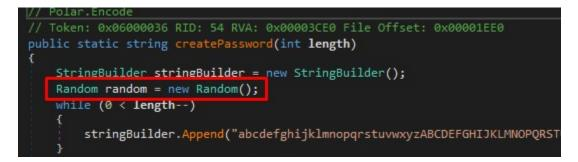
The Random function is called once, without any arguments. This call returns a random number, the seed for pseudorandom generation of which is taken from the value of the Environment.TickCount variable. This variable is 4 bytes and stores the number of milliseconds since the operating system started.
