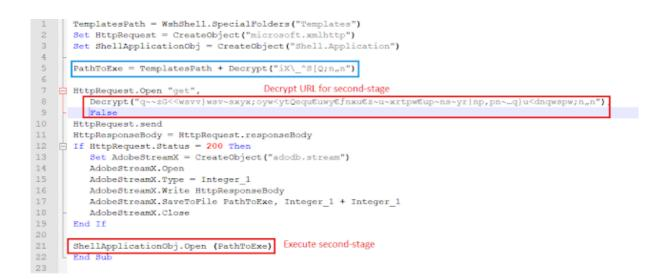
It decrypts the URL for the second-stage from hardcoded bytes, saves it to the "Templates" folder, and executes it. The traffic generated from the macro is shown below.
