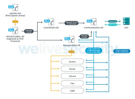
Figure 2. PipeMon IPC scheme (original PipeMon variant)
