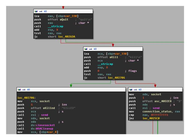
If neither "shell" or "comd" is specified by the operator, it checks if it has been instructed to sleep or terminate, otherwise it just continues to the next iteration.
