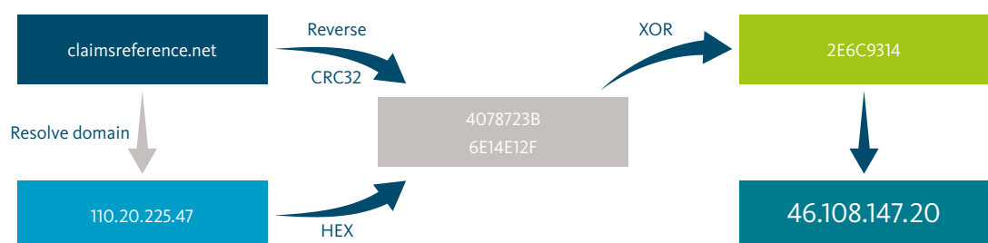
Figure 11: Conversion of a hardcoded domain to an actual command and control address
