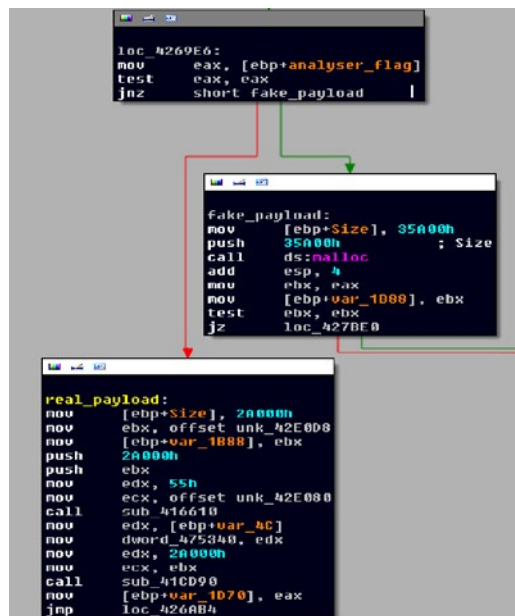
Figure 13: How the analysis flag decides between the installation of the real or fake malware
